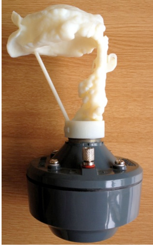
Figure 2: A 3-D print of the set of MRI images for which that shown in figure 1 is the central midline image, sitting atop its loudspeaker drive unit as used in the Vocal Tract Organ.
