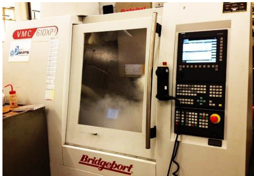
Figure 2, Bridgeport CNC milling centre used for machining experiments equipped with cryogenic cooling system
