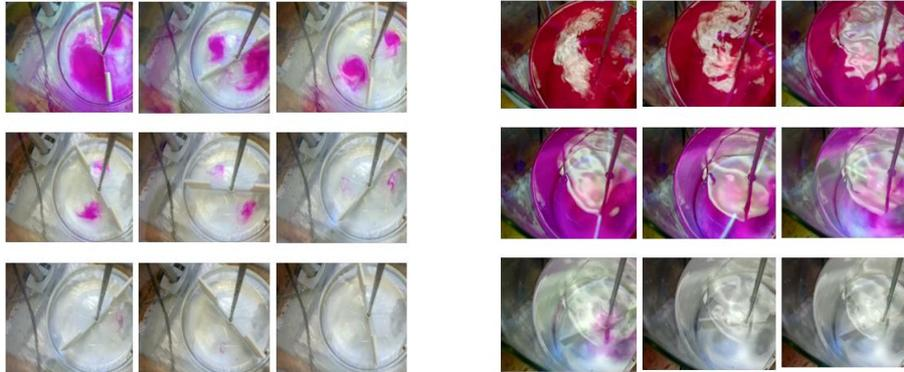
**Figure 3 - Time-lapsed photographic images throughout mixing of the decolourisation agent at (a) 25% and (b) 100% fill levels**
