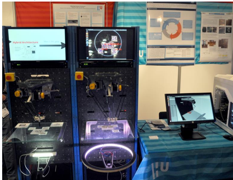
Figure 2: two equiplets with deltarobots and a 6 axis simulator on the right
