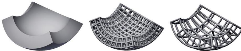
Figure 3: The energy absorbing inner liner of helmet. Illustrated are the solid block model (left), the 25% lattice structure (middle) and the 10% lattice structure (right).
