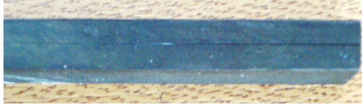
Figure 2: Composite Specimen with sampler damage of crack
