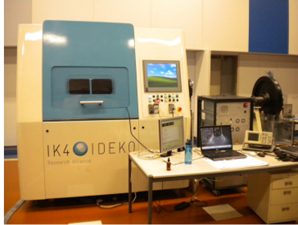
Figure 2: The in-house developed ultrafast laser ablation machine IK-Laser.
