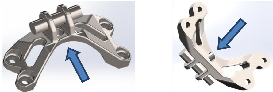
Arrows indicate the construction direction by means of ALMe
