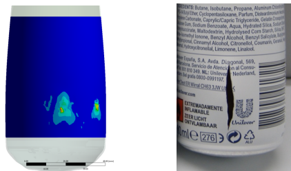
Figure 4: Burst location and shape: numerical (left) and experimental (right)
