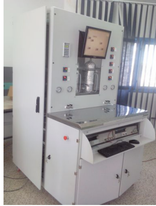
Figure 2: PEFC test station built at CRTEn.
