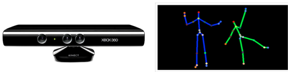
Figure 1: RGB-D camera and resulting skeleton tracking
