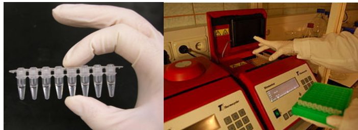
Figure 1. PCR tubes with reaction mixture placed in thermal cycler that is used in targeted DNA sequence amplification [9].
